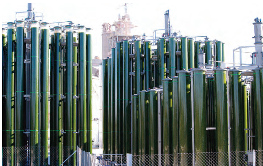
Figure 1. BFS' tested and certified (SGS) Industrial plant that absorbs CO 2 emitted from an adjacent cement factory. Plant Tour: https://www.youtube.com/watch?v=v33kNULlvs
