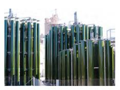
Figure 1. BFS' tested and certified (SGS) Industrial plant that absorbs CO<sub>2</sub> emitted from an adjacent cement factory.
