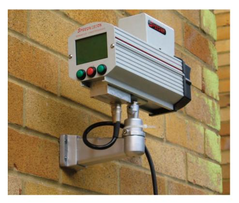
of speed violations whilst not endangering operatives standing roadside to operate the equipment. Recording of violations is to a CF card from which photographs with overlaid data can be produced using dedicated software. This has completed tests and literature will be available shortly.
