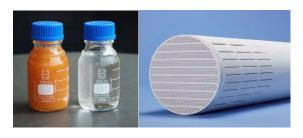
**Figure 3.** Left to right: spent filter backwash water, produced MF permeate (reused to produce drinking water), ceramic MF membrane (METAWATER Co., Ltd.)
