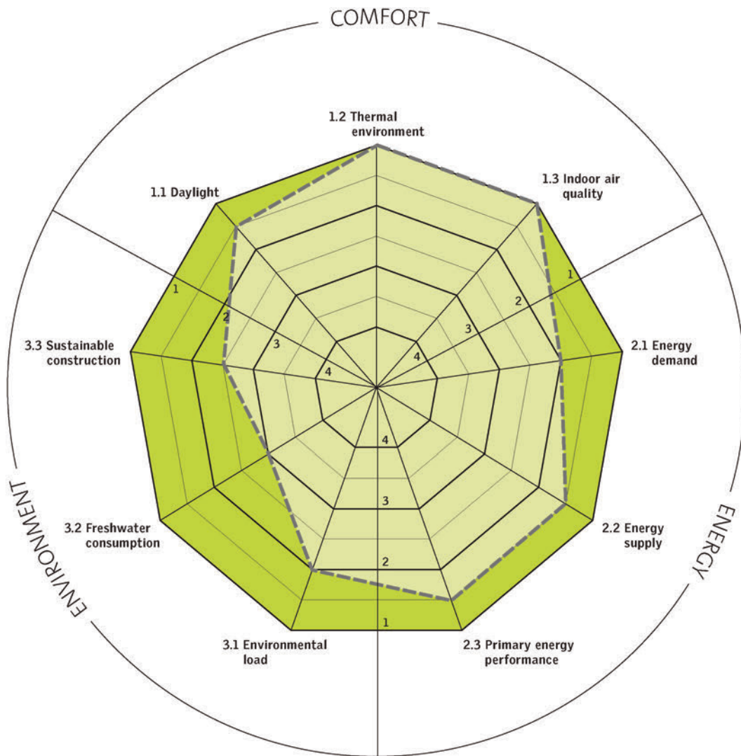
Fig 4. The Active House specifications and labelling system is very useful to communicate the Active House quality of a building project, with respect to energy, comfort and sustainability, and it can, at the same, time be used as a dialogue and performance verification tool. (see also www.activehouse.info )
