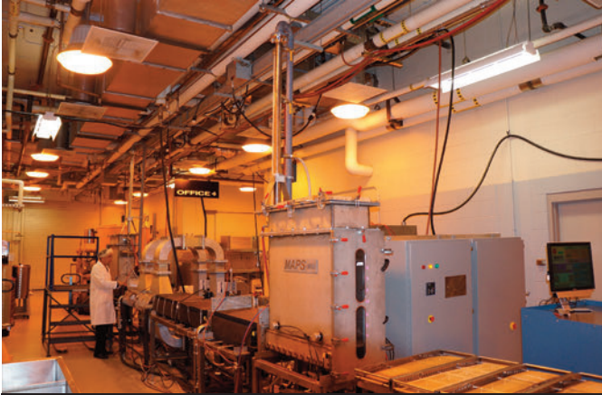
A Washington State University-led research team member works on the prototype microwave assisted pasteurization system (MAPS) unit. MAPS allows packaged foods to be safely processed more quickly and at lower cost than conventional processes
