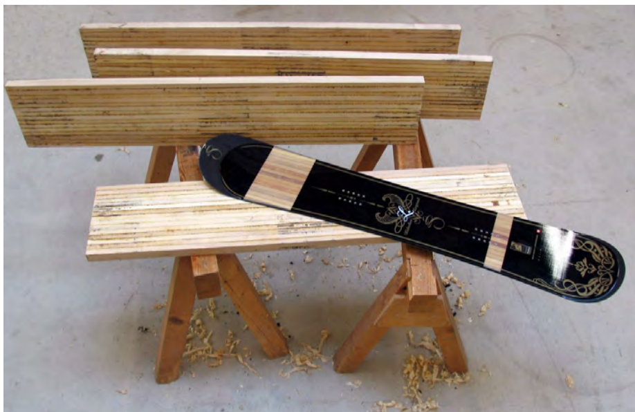
A welded snowboard core without any adhesive
