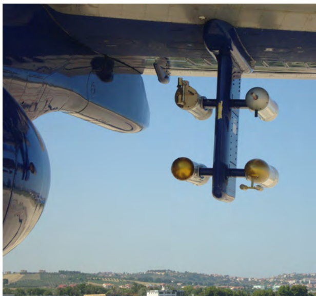
Figure 4. One of the more obvious external modifications that converts a BAe146 into the UK's FAAM atmospheric research aircraft. Underwing pylons carry a range of probes that are used for counting and sizing individual cloud droplets and aerosol particles.
