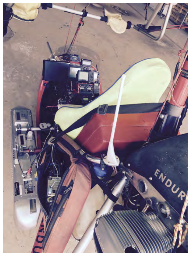
Figure 2. The pilot's seat and some of the instrumentation of the Enduro microlight operated by Karlsruhe Institute of Technology. Although small and light in weight, the aircraft is comprehensively-equipped to measure a wide range of parameters in and above the atmospheric boundary layer.
