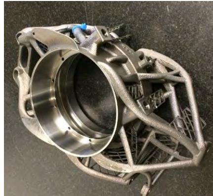
Figure 1: High stiffness and low weight titanium upright for high performance race car fabricated by AM, courtesy of Jørgen Eliassen, Revolve NTNU Trondheim
