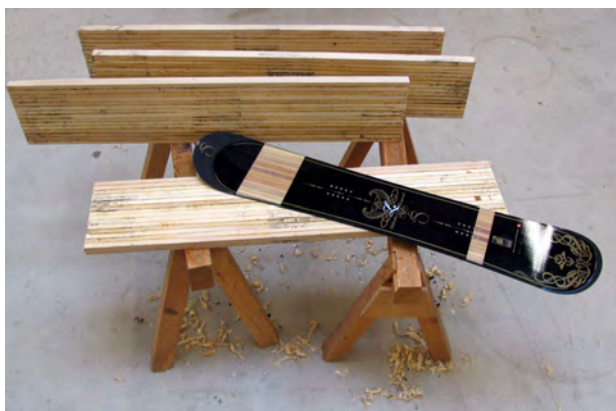
A welded snowboard core without any adhesive
