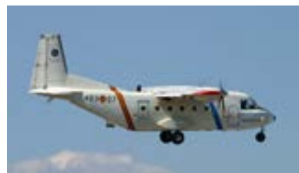
Figure 3. The CASA-212 airborne remote-sensing aircraft of INTA, Spain. This aircraft carries a range of hyperspectral imaging sensors from visible to thermal infra-red wavelengths and has also been in high demand through EUFAR Transnational Access
