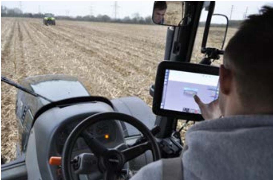
Level 2 Land-based student Ben Clothier sets up the GPS system on the driverless tractor at Wiltshire College Lackham
