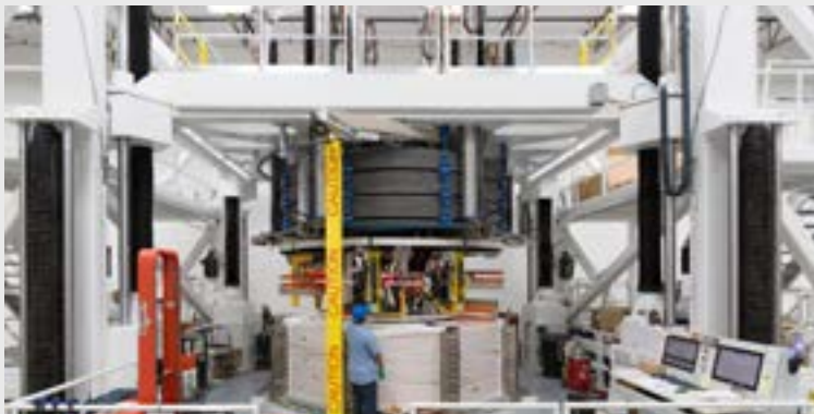
A segment of the colossal Central Solenoid magnet, "the beating heart of ITER," under fabrication at General Atomics near San Diego, California, USA.
