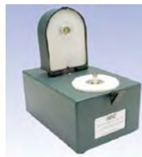
Isothermal coin cell calorimeter
