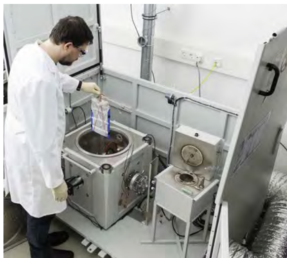
Fig.1 Insertion of a 40 Ah pouch cell into a large-size Accelerating Rate Calorimeter (ARC)
