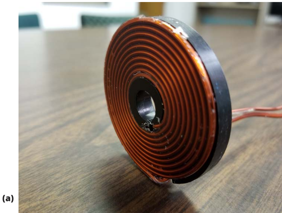
Fig. 3. The new HJ1 gas valve and pre-ionizing technique: (a) the gas valve drive coil is planar, axisymmetric, precision wound and highly reproducible. (b) The
