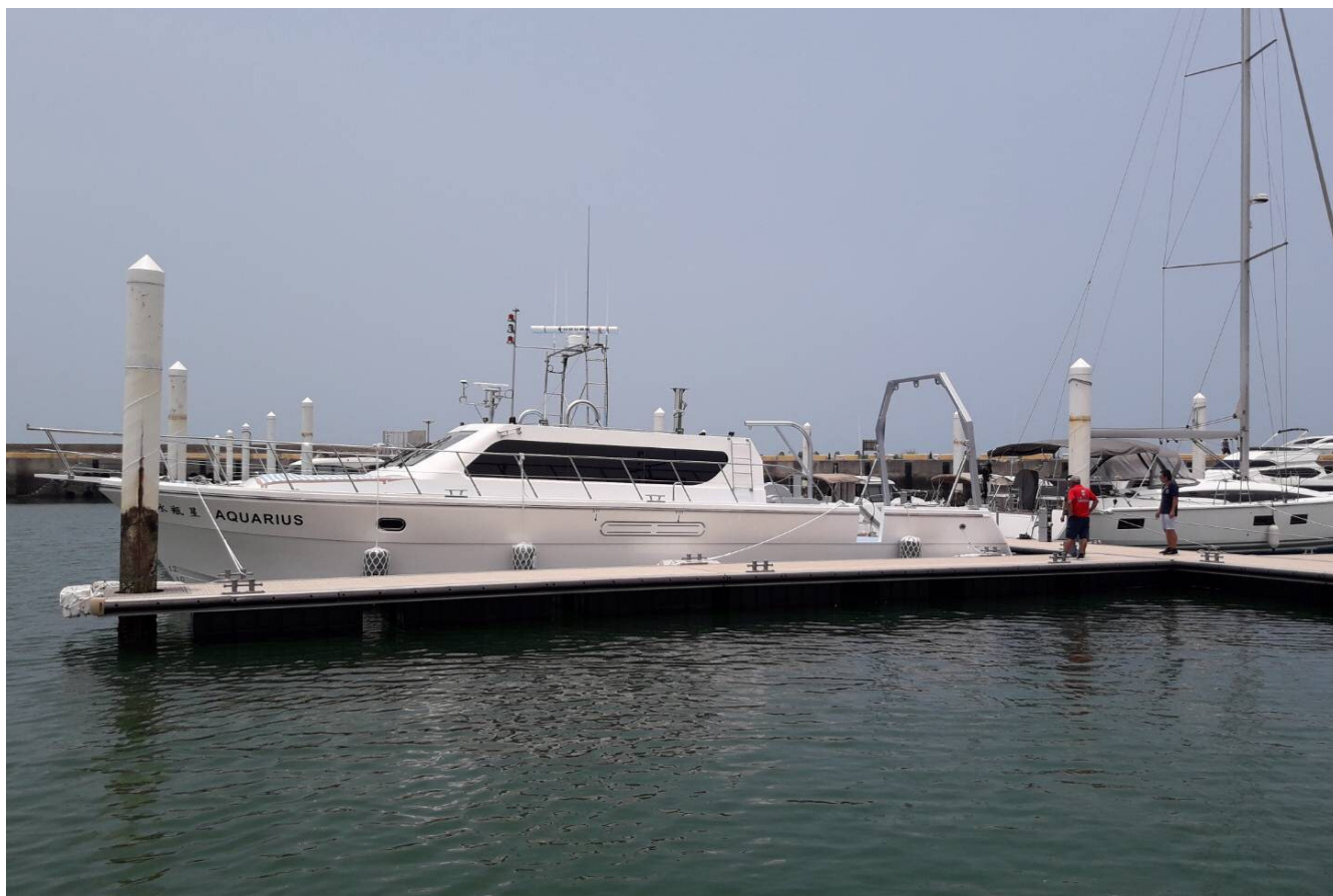
M/V Aquarius, Built in 2019, 62-foot survey vessel owned by Global Aqua Survey Limited. Equipped with multibeam echo sounders, subbottom profiler, USBL positioning system, A-Frame and 2000m cable winch.
