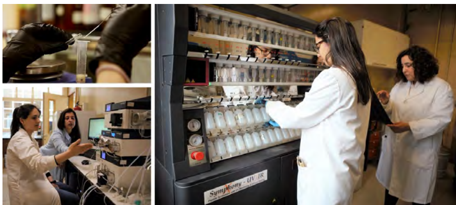
Figure 1: It took 15 years for Paula Gomes to gather the necessary means to set up and consolidate a peptide synthesis lab that evolved from exclusively manual methods (top left) to fully automated synthesis using state-of-the-art multiple-channel instrumentation (right) and purification by preparative high-performance liquid chromatography (bottom left). Setting up a large-scale peptide synthesis and purification unit able to meet the requirements of industrial partners is Gomes's next goal.
