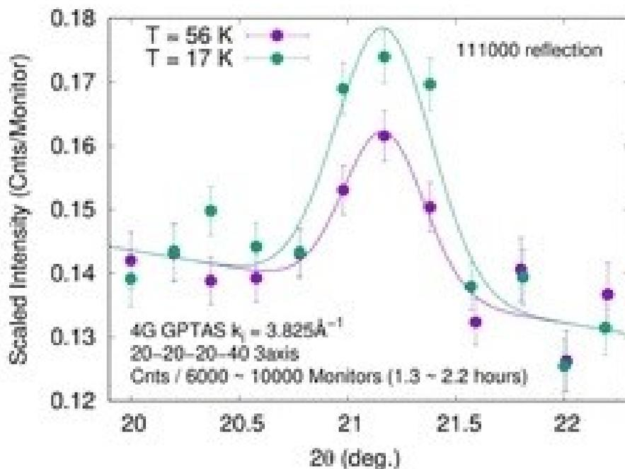
The peak profile around the 111000 reflection in the icosahedral  $\text{Au}_{65}\text{Ga}_{20}\text{Gd}_{15}$  QC at temperatures below and above the Curie temperature [13].
