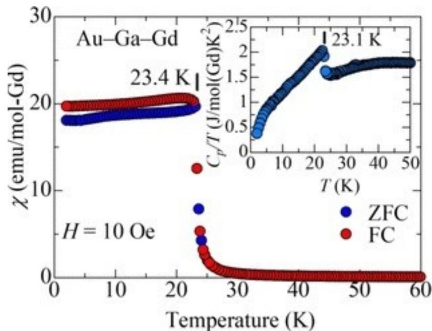
Temperature dependence of the zero-field cooled (ZFC) and field-cooled (FC) magnetic susceptibility,  $\chi$ , of the icosahedral  $\text{Au}_{65}\text{Ga}_{20}\text{Gd}_{15}$  QC measured under 10 Oe. The inset shows the temperature dependence of the specific heat,  $C_p$  [13].
