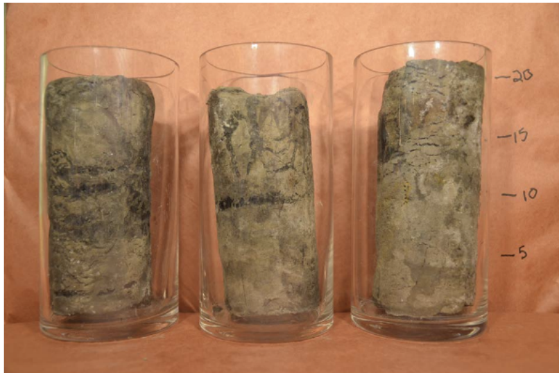
Figure 1: Three ground cores with varying ice contents before thaw, from left to right, high, medium, and low ground ice contents, respectively. Ice lenses are visible in the cores with medium and high ground ice content.
