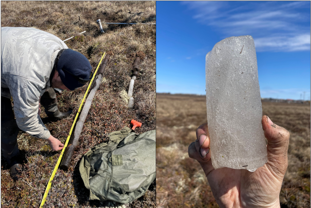
Figure 1: On right, Permafrost Grown team member Mikhail Kanevskiy analyzes a recent collect core collected from an ice wedge trough in Bethel, AK. On left, Mikhail holds a core section of wedge ice that will cause thaw subsidence if the permafrost it's in degrades.
